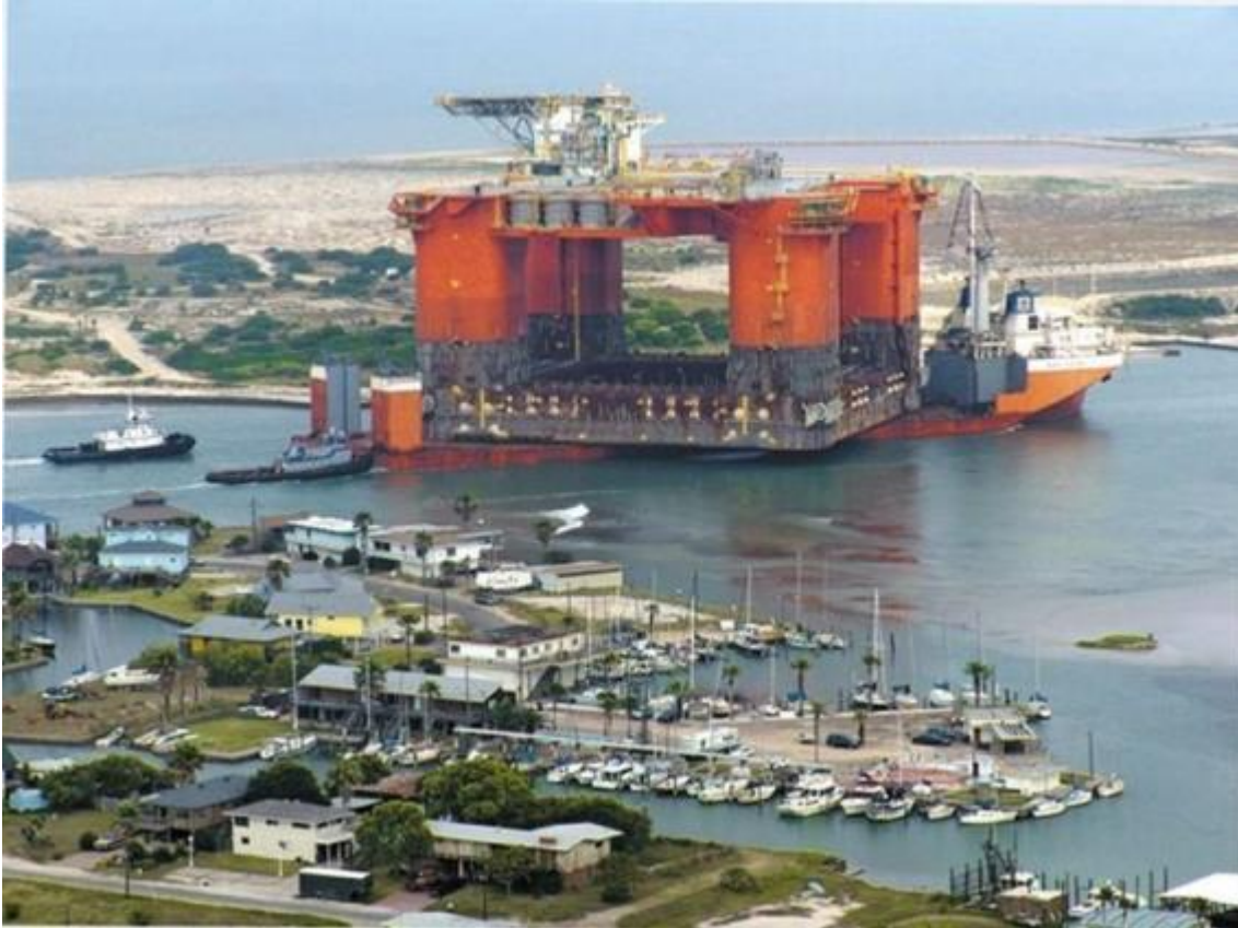
Figura 6b – Transporte de plataforma por um HLV ( http://www.amusingplanet.com/2012/05/heavy-lift-ships-and-their-impossibly.html )
